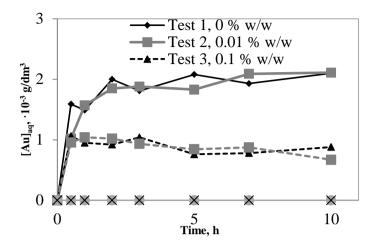
Fig. 2. Gold concentration in solution as a function of time during halide leaching. Additional organic carbon concentrations in non-preg-robbing ore were from 0, 0.01, 0.1, 1, 5 and 10% w/w in Tests 1, 2, 3, 4, 5 and 6, respectively
